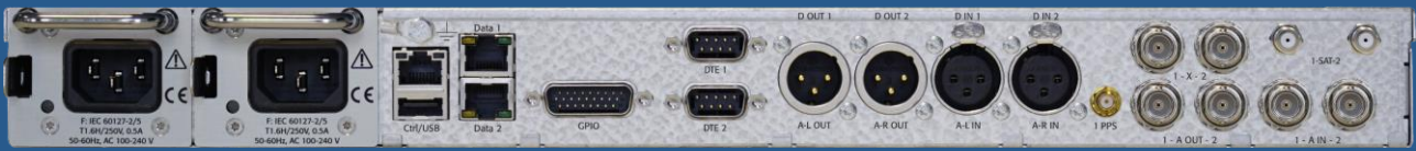
Back panel of MPX-1g. MPX-d back panel is reduced to output interfaces.
